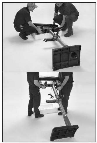
Figure 12. Tilting drill press upright.
